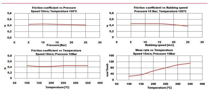
Rubbing speed, temperature and pressure are related. Changing any values will change other. The values shown represent typical conditions, but are not ultimate limits of the material.
